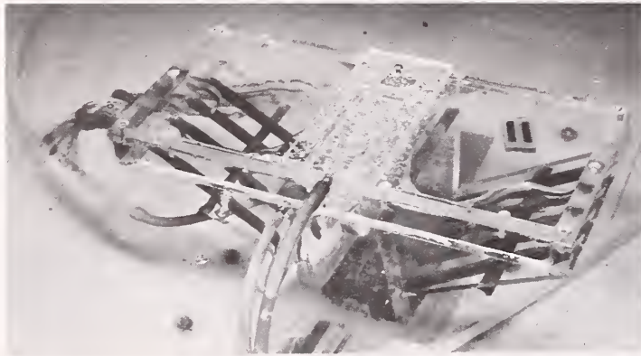
Figure 10.—Vents open, head 2.95 ft, discharge 457 c.f.s. Small vortex at left upstream corner of antivortex plate, air trapped under upstream outside corners of antivortex plate, splash on underside of antivortex plate over drop inlet, weir control, drop inlet partly full, air being entrained by nappes.
